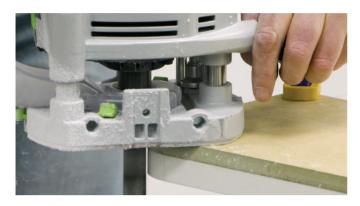
We recommend that all cuts are finished with a router as it will leave less tooling marks than other methods. When cutting with a router or circular saw, the cut should be made in several passes to prevent overheating. We recommend cutting 20mm thickness Mirostone using 4 consecutive passes. The first at 5mm depth, the second at 10mm depth, the third at 15mm depth and the final pass should be greater than 20mm to ensure the cut is complete.
