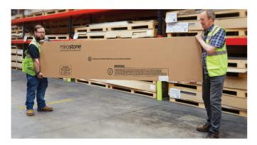
Before commencing any fabrication or installation work, inspect your Mirostone solid surface products and ensure you are satisfied that there are no defects, for example: colour matching defects.
