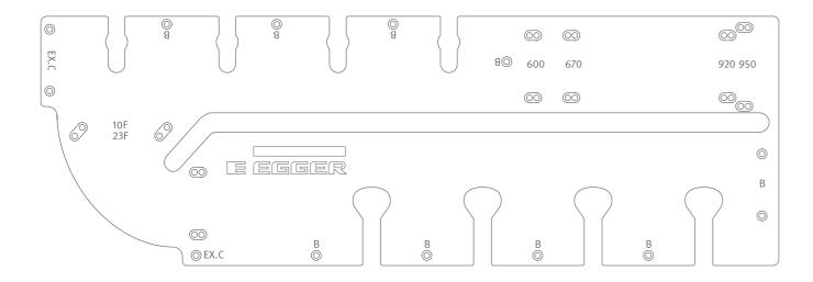
This jig can be used to fit 90° corners for all EGGER worktops. It has fixed worktop width settings of 600 mm, 670 mm, 920 mm and 950 mm. However, it can be used to cut worktops of any width smaller than the maximum capacity of the jig (950 mm) using appropriate shims and spacers.
